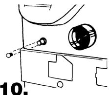
Remove the red caps from the gas pipes.
